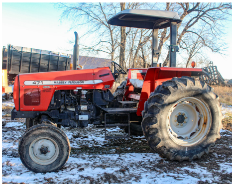
Massey Ferguson 471 Diesel Tractor, Wide Front, 3 Point, Dual Hydraulic, Canopy, 3748 One Owner Hours, Ser# 9363BM28015
